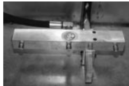
A special reciprocating nozzle head provides total coverage for a variety of screen sizes.
